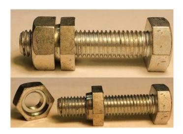
Another two-nut design in present use is the Tracksure/Wheelsure product. The special bolt which is used has a smaller left-hand on the end. The main nut is tightened fully and then locking nut, having a left-hand thread) is applied until it tightens against the original nut. A steel locking cap pushes down over both the original nut and the locking nut, the cap being held in place with a spring clip.
